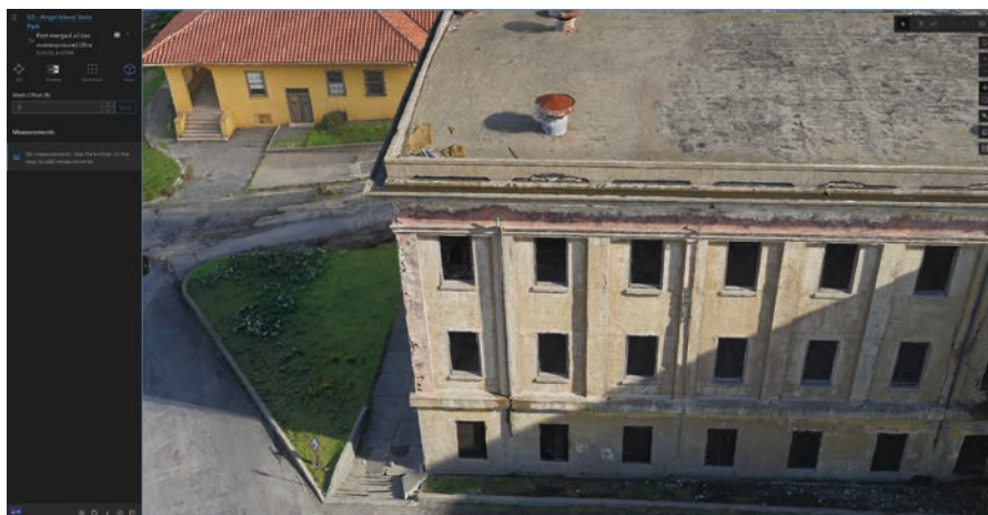
↑ A drone-acquired 3D mesh of historic buildings on Angel Island State Park in Northern California.
