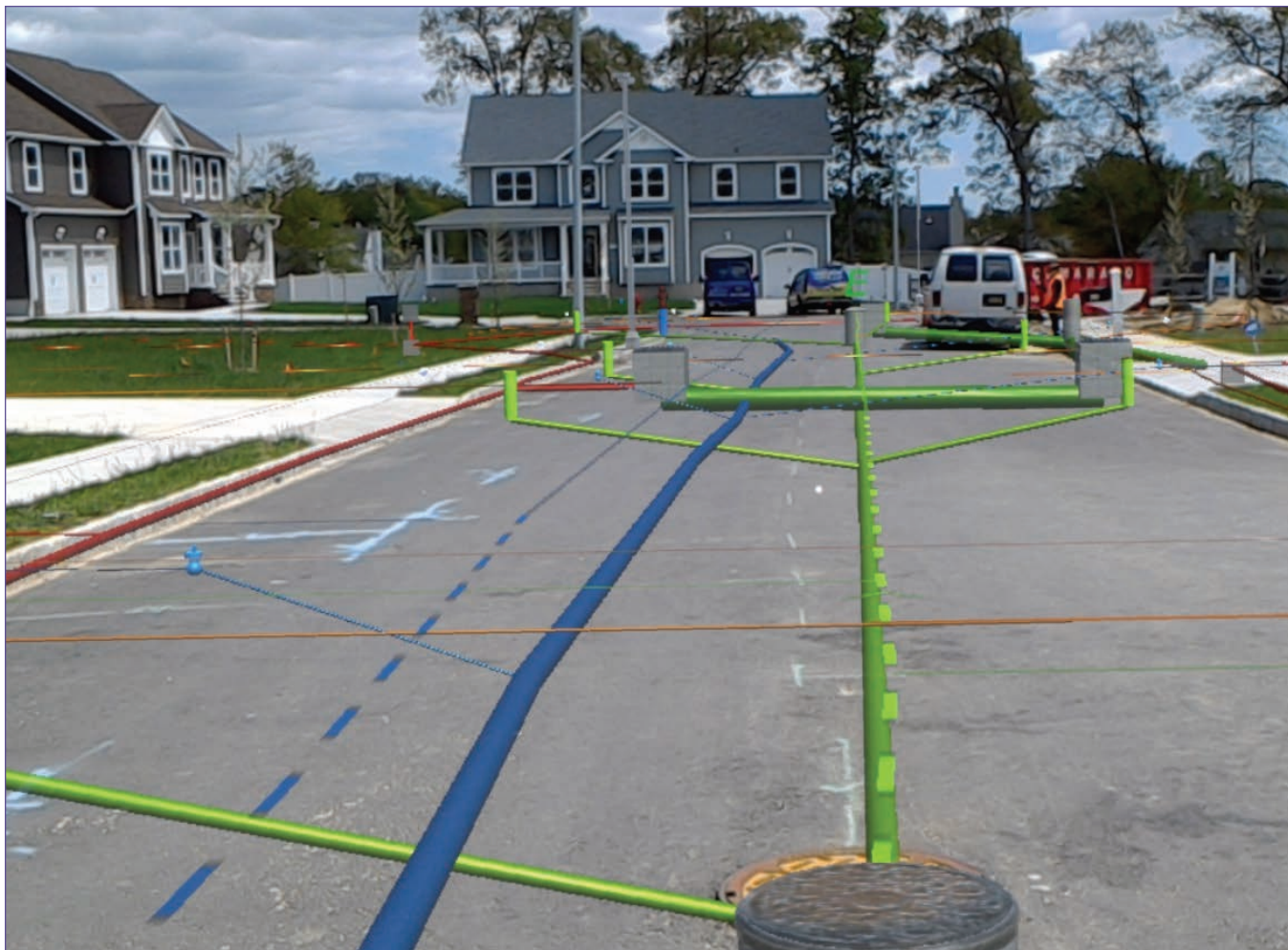
↑ Staff at TRMUA use Microsoft HoloLens and an app developed by Esri partner Meemim, Inc. to visualize ArcGIS feature data describing TRMUA's underground utilities.
