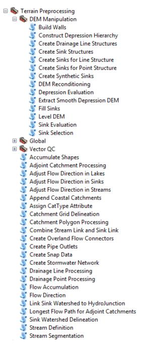
Figure 1. Arc Hydro Terrain Preprocessing toolset (Arc Hydro Tools Python toolbox)
