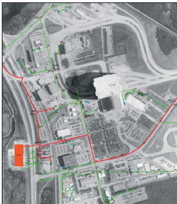
A trace of a specific electrical feeder through the Vehicle Assembly Building area.
