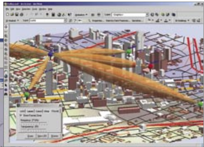
Figure 2. GIS helps engineers plan wireless networks using wave propagation and line-of-sight analysis and visualization, as shown here.
