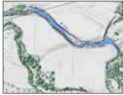
Existing riparian canopy and topography within a potential planting site based on lidar data. The current canopy is used to model the incoming solar radiation under preproject conditions.
