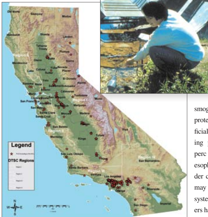
Inset: A water sampler uses GPS to attach coordinates for mapping attributes in GIS. Above: DTSC uses ESRI ArcGIS to produce the map of perc detections in public water supply wells. (Data is from the California Department of Public Health Water Quality Database.)
