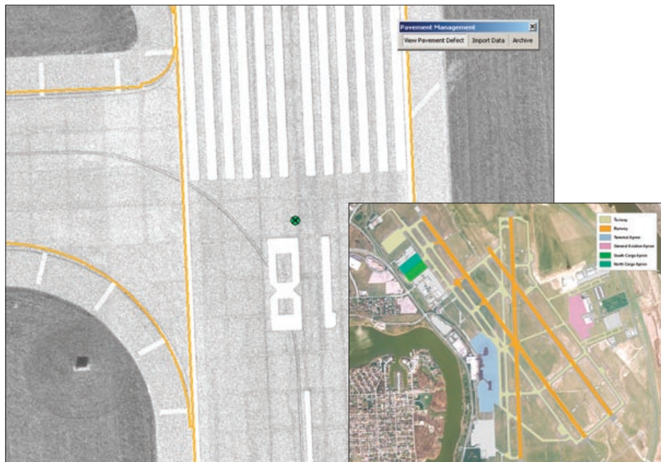
A mobile GIS solution allows Eppley Airfield in Omaha Nebraska to map and document runway surface defects.
