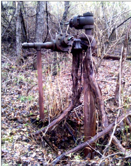
↑ Remains of a Historic Well That Was Abandoned and Overgrown by Brush and Trees
