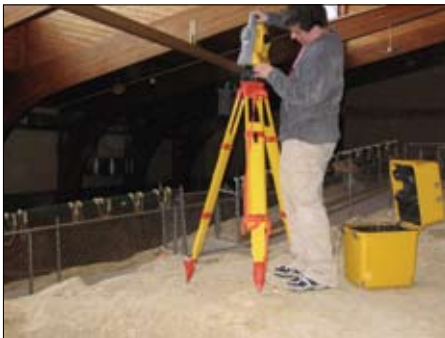
The Trimble 5600 robotic transit being mounted to its tripod
