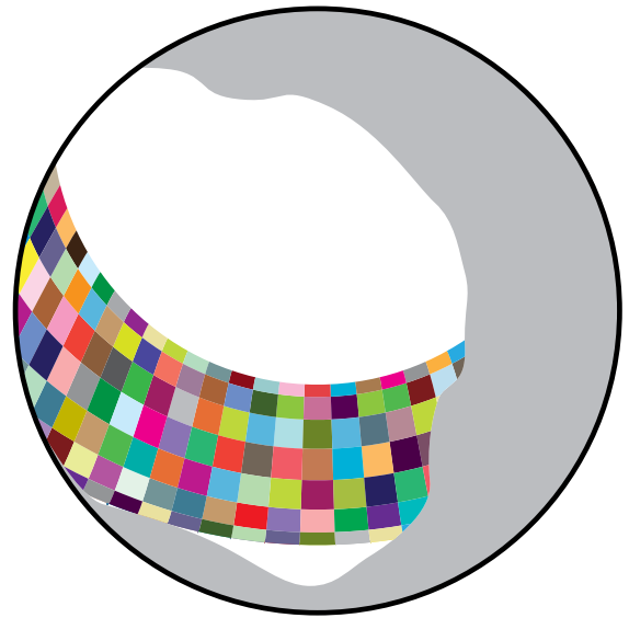
The sunmap is further overlaid with the calculated viewshed to calculate the direct solar radiation.
