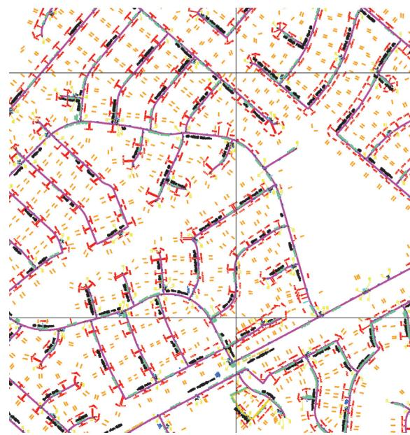
↑ The GIS team converted hundreds of MicroStation-based water/sewer map layers, such as this one, into GIS-based, spatially accurate map files that support the asset management system.
