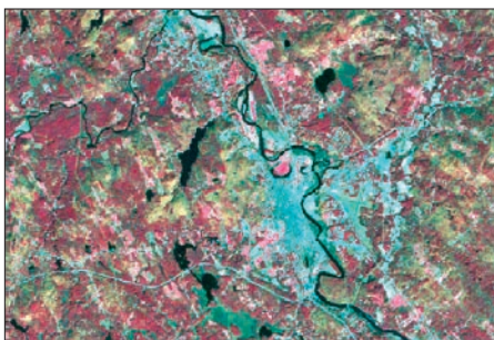
Landsat 7 image view with a false color band combination (Band 4, red; 3, green; 2, blue). Data courtesy of the University of New Hampshire, EOS-WEBSTER Earth Science Information Partner.
