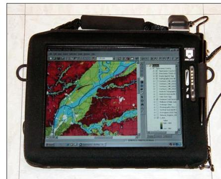
GIS loaded on a ruggedized tablet allows users to view specific data in the field to determine soil characteristics and perform analysis.
