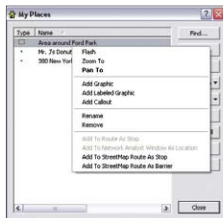
Right-clicking on a location in My Places invokes a context menu with navigation, display, and other choices.
