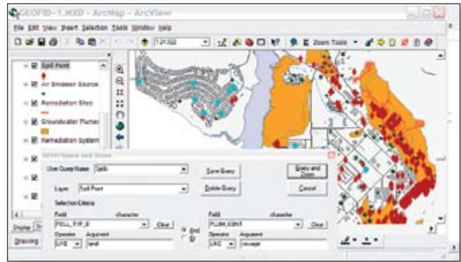
Example of a user-defined “zoom” that can be saved, edited, and reused
