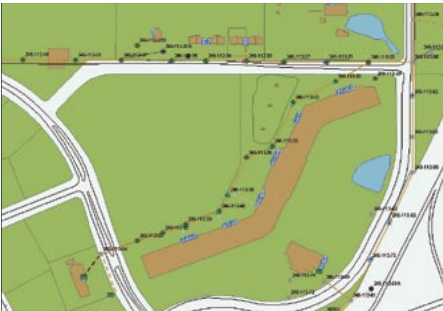
CAD data is placed into a seamless database so that the existing tiled CAD data can be made to perform seamlessly inside the GIS.
