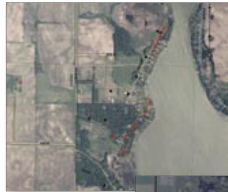
Figure 2 Outage status and response is coded by color. No power and not dispatched are red. No power and dispatched are blue. Restored power from an outage is green. Personnel click on a blue section to see which truck has been dispatched to the site.
