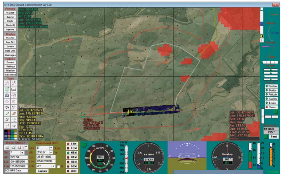
↑ This is the GIS-based ground control and flight operations interface. As the UAV flies its mission, the flight lines are tracked and adjusted as needed. Right: The RQ-84Z AeroHawk UAV, shown in flight, is used by Flightline Geographics to capture FMV data at a low cost.
