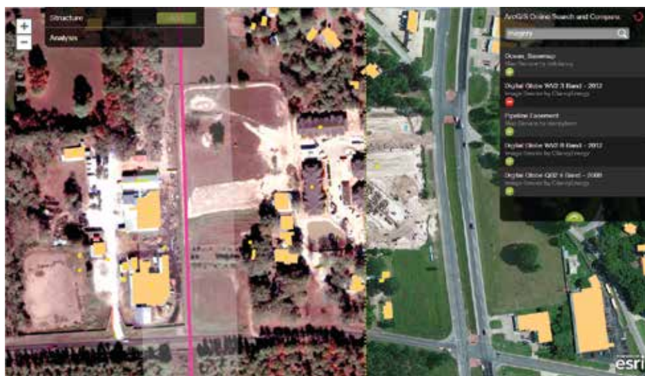
↑ Underground pipeline and asset data added to satellite imagery and lidar improves analysis.
