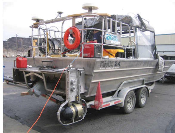
Idaho Power has a boat equipped with a wide range of sensors to measure and monitor the health of the Snake River.
