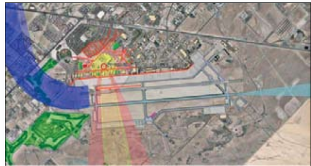
Notional aircraft incident at Nellis AFB, demonstrating approach and departure corridors, plume modeling, traffic control, and building evacuation status
