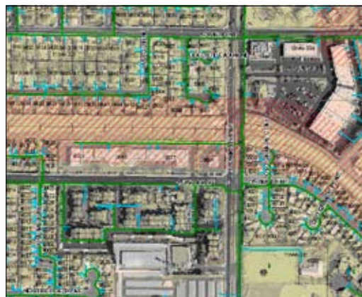
Task assistant tools have empowered New Mexico Gas Company designers with the ability to map designs for new construction and maintenance.
